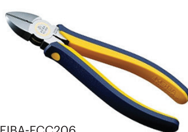
KEIBA-FCC206 Side Cutter 160mm Keiba • High Grade Series with high- class non-slip handles. • Cutting capacity: hard wire diameter 1.8mm, soft wire diameter 2.3mm
