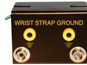
POSH1241 ESD Grounding Box 2x4mm Banana • Workbench bonding points • Can be used by two people simultaneously. • No resistor, ground cord with 4mm ring terminal • Ground bonding point, for 2 x 4mm banana plug and 2 x 10mm snap
